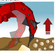
nelled into a double nitrogen accumulator. Thanks to a pressure gauge it is possible to set the release force of all the shanks.
