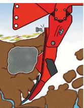
When the maximum load is exceeded, the breaking of the bolt allows the shank to be raised, avoiding possible damage to the shank and the frame.
