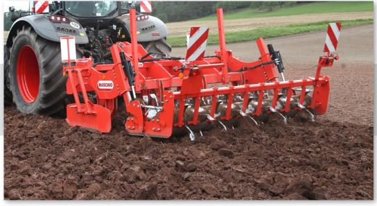
ARTIGLIO and ARTIGLIO HYDRO can be hitched to tractors with a three-point attachment of CAT 3, 4N ISO + 3 and 4N ASAE.
